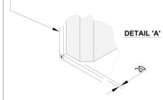
Lining elements set back in casing by 20mm and provided with aerodynamic fairings on inlet and outlet as shown. However if item has non-standard elements refer to Attenuator Model Code Definitions for details.
