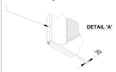
Splitter elements set back in casing by 20mm and provided with aerodynamic bullnoses on inlet and outlet as shown. However if item has non-standard elements refer to Attenuator Model Code Definitions for details.
